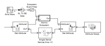
Alternatively, you might be able to address the problem by using an attribute directly instead of by using the signal output of a Get Attribute block.
